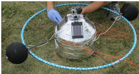
Figure 10: Final payload assembly with field probes
